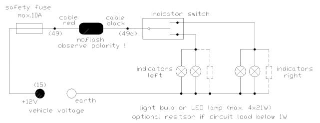
ATTENTION! THE MINIMAL SUPPLY CABLE WIDTH IS 0,75MM<sup>2</sup>. YOU MUST FUSE THE +12V POWER SUPPLY CABLE WITH A 10A SAFETY FUSE. IF THE DEVICE WILL BE USED WITHOUT FUSE, DAMAGE AT THE CONNECTING CABLE OR THE MO.WAVE ITSELF CAN CAUSE A SHORTCUT AND A CABLE FIRE. THERE MAY BE A RISK OF YOUR LIFE! IF YOU ARE NOT CAPABLE TO CONNECT THE DEVICE PROPERLY, LET THE PROFESSIONAL MOTORCYCLE TECHNICIAN DO THE JOB.
